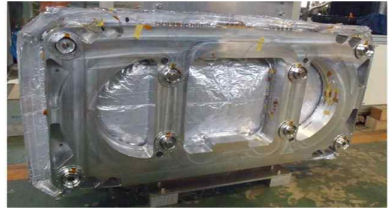
Fig.2 Assembled REBCO coil for Maglev [8]
