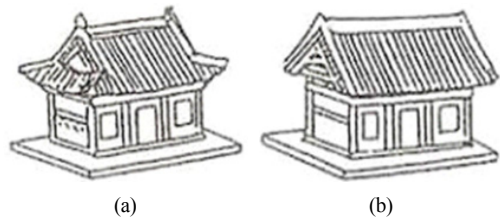
Fig. 2. Sketches of hanok structures showing (a) a Mat-bae roof and (b) a Pal-Jak.
