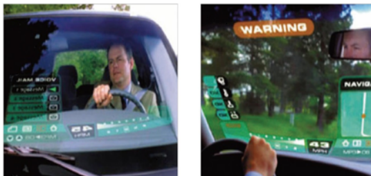
Fig. 1. AR example - Driving information displayed on the windshield.
