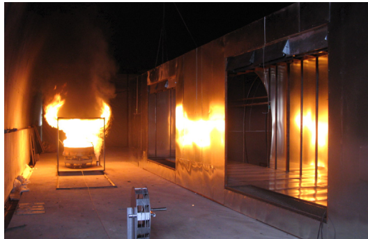
Fig. 9. View of a full-scale fire test (during test)
