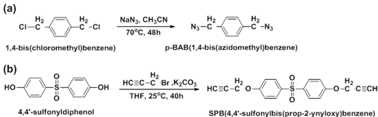
Fig. 3. The reaction scheme of the novel toughening agent monomers, (a) p -BAB and (b) SPB.
