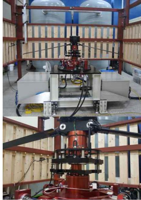
Fig. 7. Manufactured tipjet rotor test equipment
