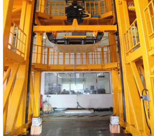
Fig. 19. Free drop facility and testbed
