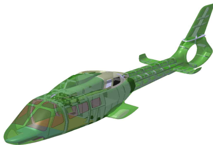
Fig. 2. Conceptual design and structural layout of testbed helicopter
