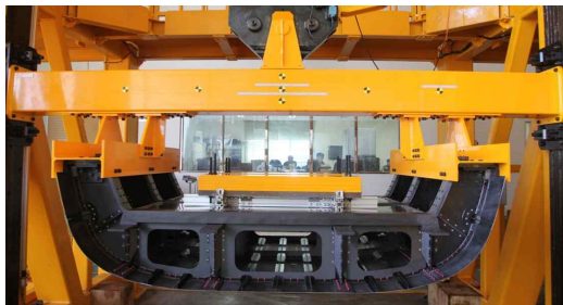
Fig. 18. Composite crashworthy subfloor testbed
