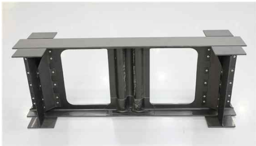
Fig. 12. Test specimen of crush web assembly
