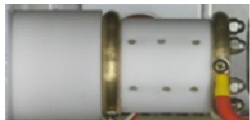
Fig. 15. Fabricated spark gap of the TG.
