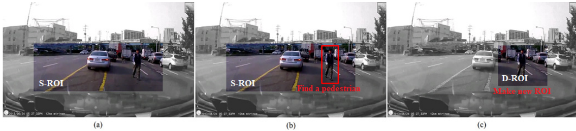
Fig. 1 Example of operation of dynamic region of interest (D-ROI) for pedestrian recognition method
