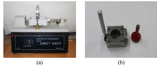
(a) Direct Shear Tester (b) Shear Box Fig. 1. Apparatus of Direct Shear Test
