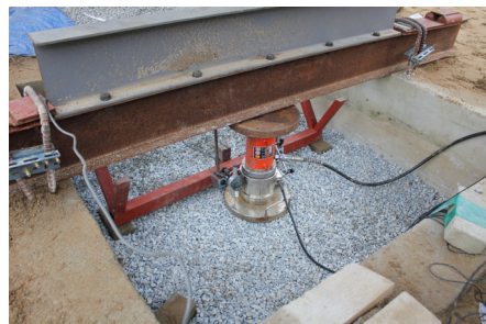
Fig. 9. Plate load bearing test
