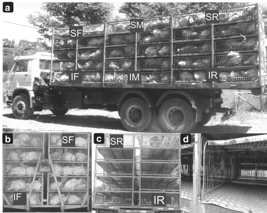
Fig. 2 a ) Photograph of the truck container side loaded with turkeys showing the strategic locations of the data-loggers: SF: Superior Front, IF: Inferior Front, SM: Superior Middle, IM: Inferior Middle (IM), SR: Superior Rear and IR: Inferior Rear. b ) Photograph of the truck container front-view showing the positions of the columns and the data-loggers (dark gray). c ) Photograph of the truck container rear-view showing the positions of the columns and the data-loggers (dark gray). d ) Photograph showing the positions of the data-loggers in the transport cage
