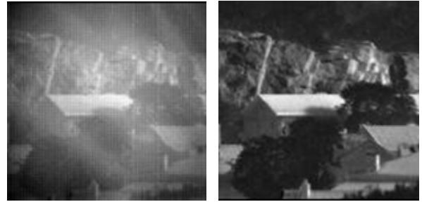
Fig. 17. Outdoor image before and after non-uniformity correction
