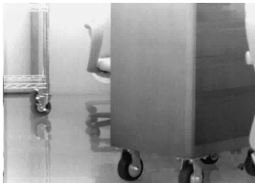
(b) Non-uniformity correction image by defocus and offset value correction based on space filter
