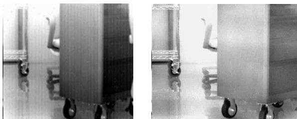
(a) Original image and non-uniformity correction image based on image by defocus
