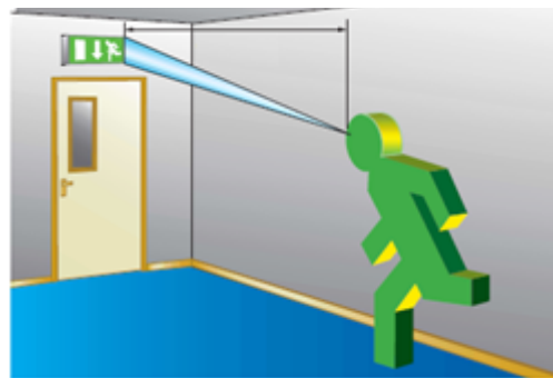
Figure 3. Emergency Exit Sign perceivable View Point
