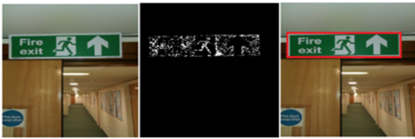
Figure 7. Emulated Object Detection Result Using CAMShift Algorithm
