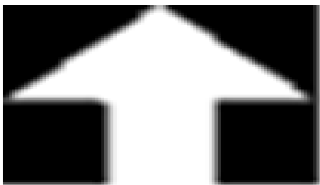
Figure 9. Extracted Sign Direction Arrow Using Template Matching
