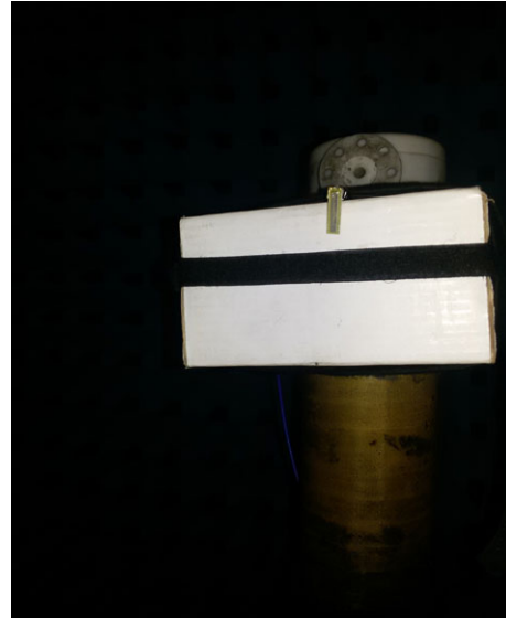
Fig. 7. Anechoic chamber testing of the fabricated antenna.
