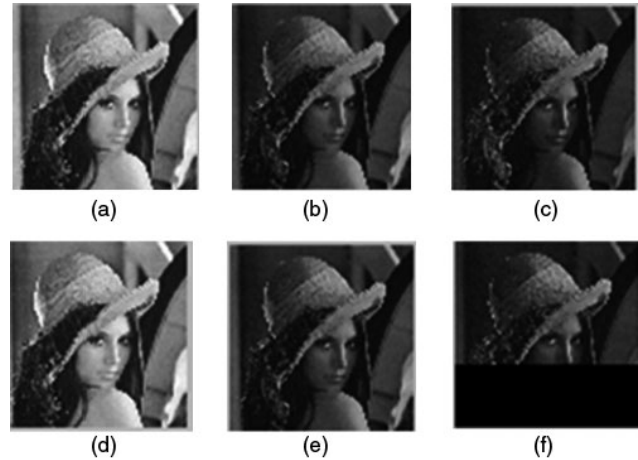
Fig. 3. Black pixels show the lost packets due to a timeout event during transmission: (a) original (red), (b) original (green), (c) original (blue), (d) received (red), (e) received (green), and (f) received (blue).
