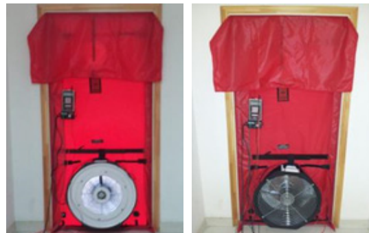
Fig. 2. Depressurization (left) and pressurization (right) mode of blower door test.
