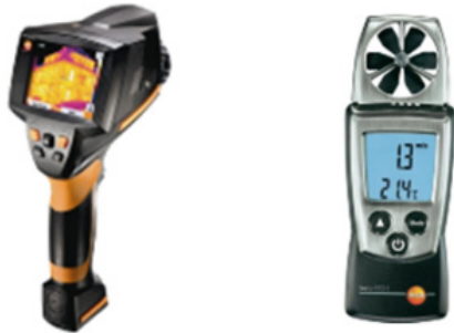
Fig. 3. Infrared camera (left) and vane anemometer (right).
