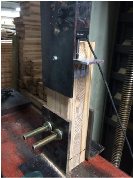
Fig. 1. Test set-up of single shear CLT-to-steel connection.
