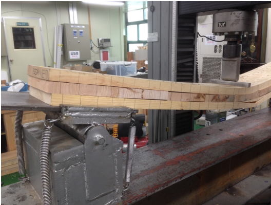
Fig. 6. Failure of a nail-jointed cross-laminated timber.
