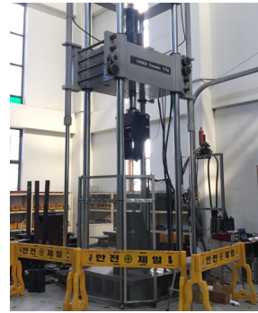
Fig. 1. 1,000 kN UTM at KICT
