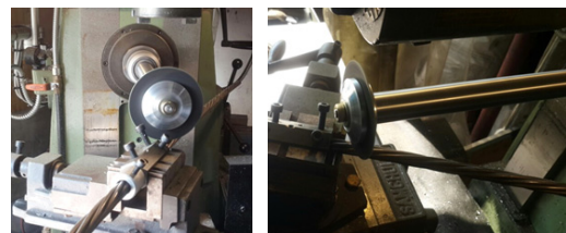
Fig. 3. Artificial Damage using milling machine on 7-wire strand
