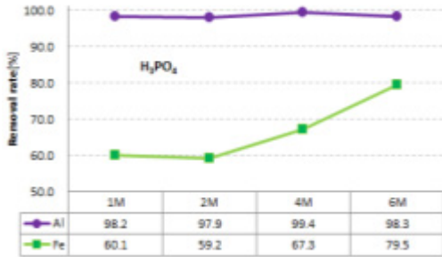
Fig. 3. Fe and Al removal rate after leaching with H 3 PO 4
