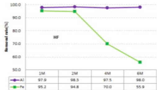
Fig. 6. Fe and Al removal rate after leaching with HF
