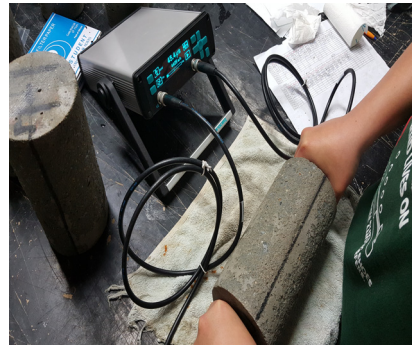
Fig. 7. Ultrasonic velocity method
