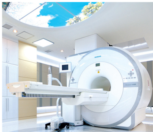
Fig. 1. PET-MRI brings the best of both worlds of PET that can diagnose liver cancer by detecting biochemical changes in the body through glucose metabolism, and MRI that can observe in high resolution soft tissue such as the liver. The integrated PET-MRI used in this study allows the artifact due to movement to be minimized as the subjects lie done to have the PET and MRI taken simultaneously. This also helps to shorten the test time which leads to better diagnosis accuracy.
