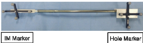
[Fig. 9] Intramedullary nail with attachment of IM Marker and Hole Marker
