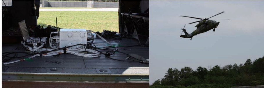
Fig. 7. GPS/INS mounted on an UH-60 helicopter for flight tests
