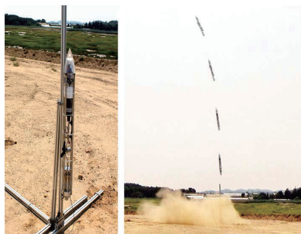
Fig. 7. Sounding rocket installed on the launch pad (left) and flight testing (right)
