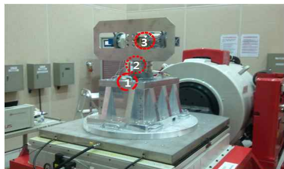
Fig. 15. Sine sweep test(x-axis), input: location 1; response: location 2 and 3
