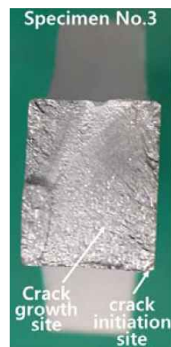
(c) Specimen No.3 crack initiation and crack growth sites
