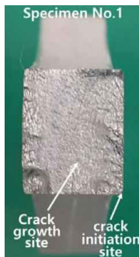
(b) Specimen No.1 crack initiation and crack growth sites
