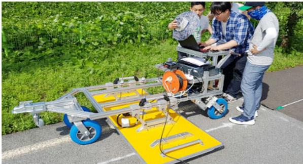
Fig. 15 Step Frequency Type GPR Testing
