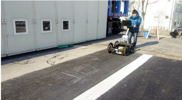
Fig. 14 Impulse Type GPR Testing
