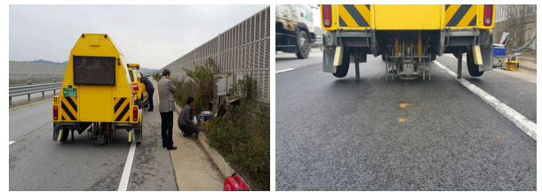
Fig. 5 FWD Test and Collecting Deflection Data
