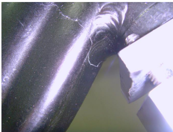
Fig. 5. Crack by horizontal load.
