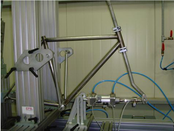
Fig. 2. Horizontal fatigue test (Road bicycle).
