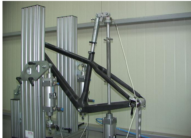
Fig. 3. Vertical fatigue test (Mountain bicycle).
