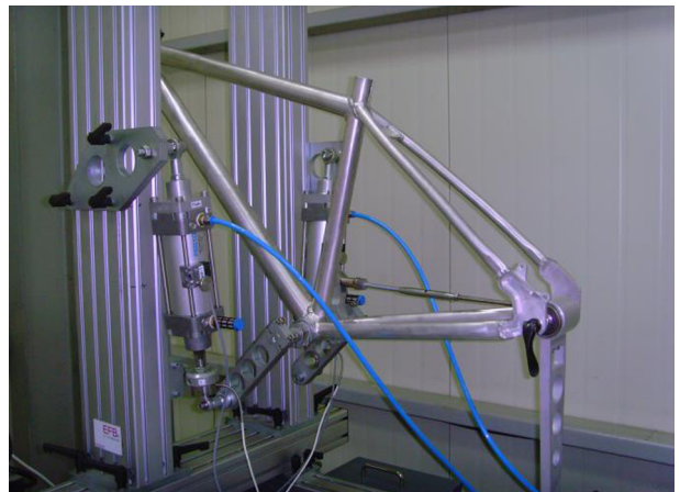
Fig. 1. pedaling fatigue test (Mountain Bicycle).
