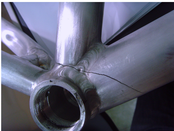
Fig. 4. Crack by pedaling Load.
