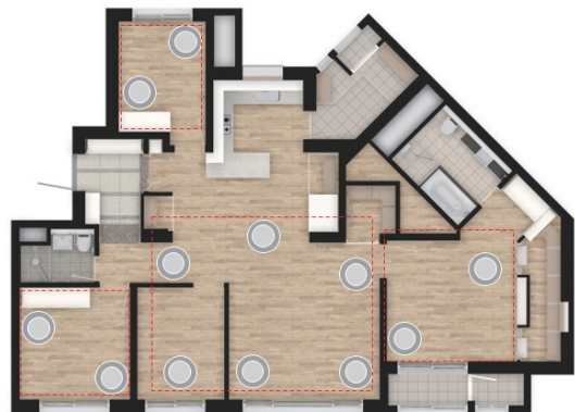
[Fig. 2] Apartment structure and diffuser location
