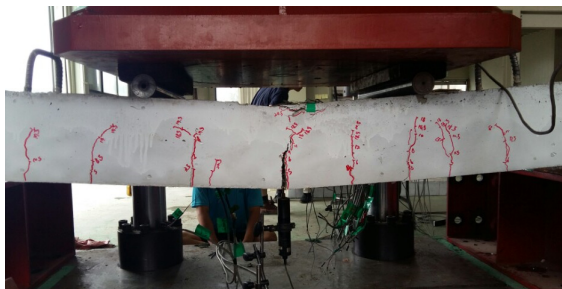
Fig. 4. Crack patterns at failure
