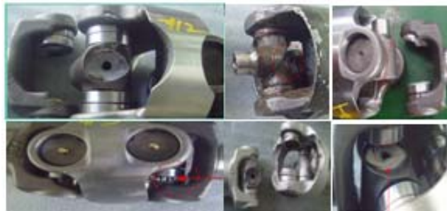
(b) Failure of the drive shaft
