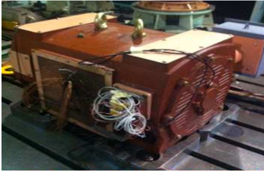
Fig. 7 Fixed model test setup for modal test
