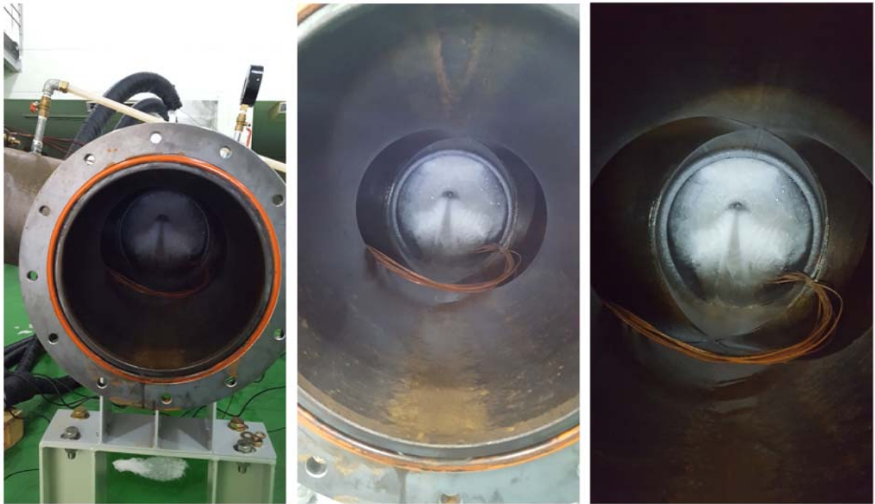
Fig. 5. Ice-Plug for freezing seal isolation in pre insulated heat transport pipe(300A) using in KDHC
