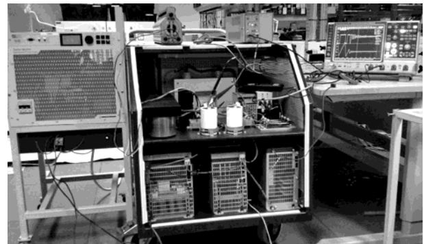
Fig. 15. Test system. The S120 MM module is on the bottom left of the cart. The inductors and output capacitors are on the top.
