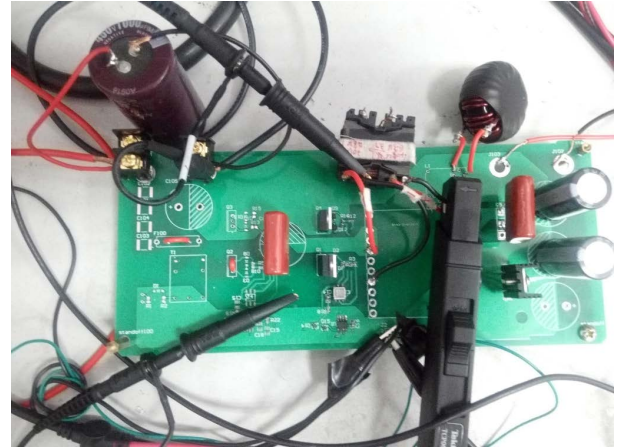
Fig. 8. Photograph of an experiment prototype for the proposed converter.
