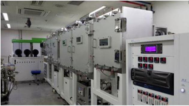
[Fig. 6] Photograph of a roll-to-roll OLED deposition equipment.
