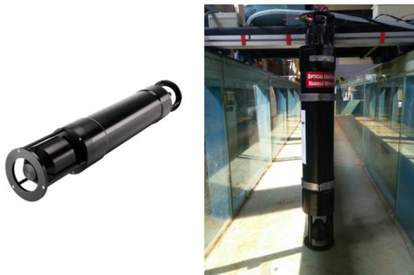
Fig. 3. Installation of Sequoia LISST-100X in the Laboratory Flume
