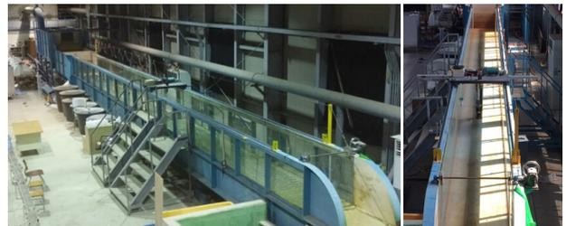
Fig. 1. Laboratory Flume to Test Hydroacoustical Characteristics in Terms of Estimating Suspended Sediment Concentration Based on SNR Observation as a Surrogate, Where LISST-100X was Utilized for Validation and Establishment of SNR-SSC Relation
