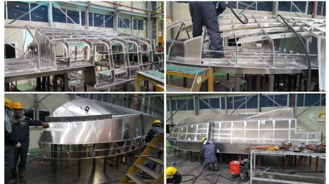
Fig. 4. Production process of waterjet net boat.
