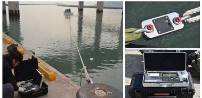
Fig. 9. Bollard pull test for net boat.
