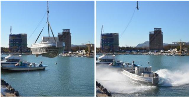
Fig. 5. Drop test for net boat.
