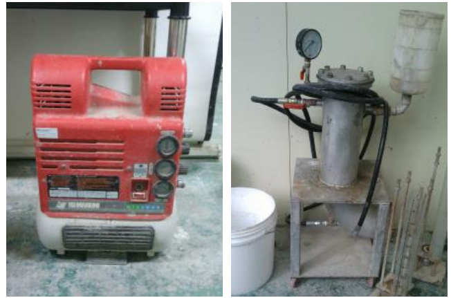
(a) Air compressor (b) Injection equipment
