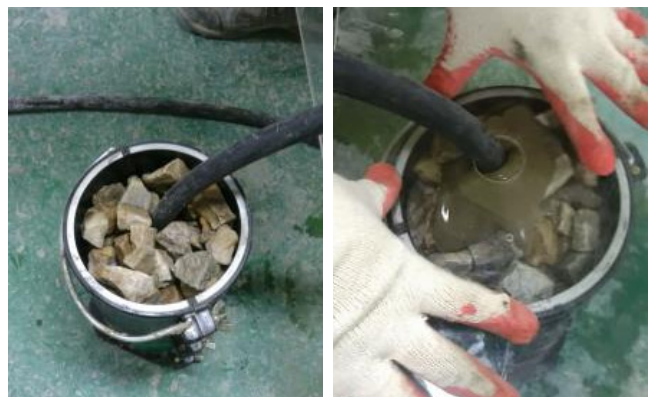
(a) Fill with aggregate (b) Grouting
