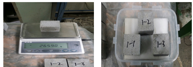
Fig. 4 Photograph of freeze-thaw test
