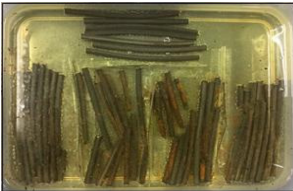
Fig. 4 Rust removal through citric acid solution
