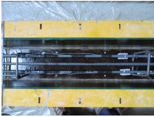
Fig. 5 Location of steel strain gauges
