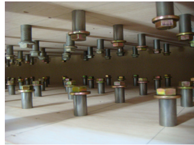
Photo 4 Inside of wall specimen
