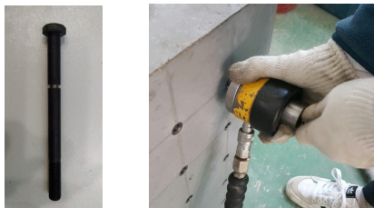
Photo 2 Break-off bolt and Simplified pullout test for high strength concrete
