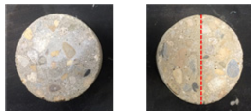
(a) Normal concrete (b) Cold joint concrete
