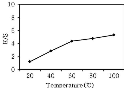
Fig. 1. Effect of dyeing temperature on the K/S values of wool fabrics dyed with *Corydalis Tuber* extract.
