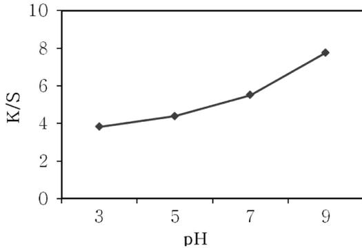
Fig. 4. Effect of dyeing pH on the K/S values of wool fabrics dyed with *Corydalis Tubor* extract.
