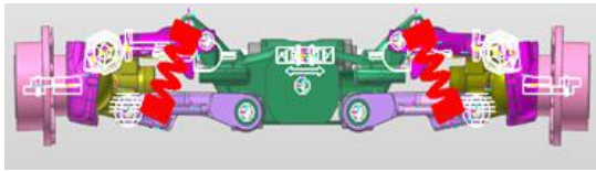
Fig. 3 Dynamic analysis model for tractor front axle suspension system
