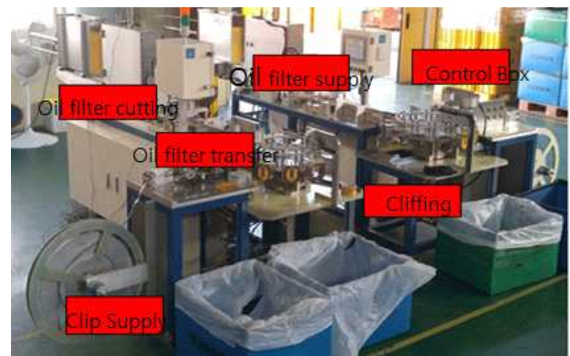
<Fig. 3> oil filter clipping automation configuration
