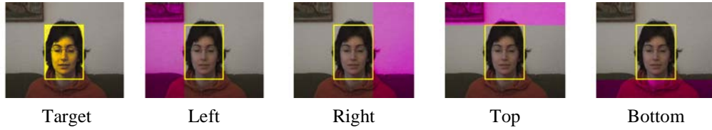
Fig. 2 (a). Layout of the target and the surrounding used for estimating joint probability distributions for the target enhancement and background suppression.
