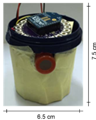
Fig. 13. Sensor node model with on-board sensors
